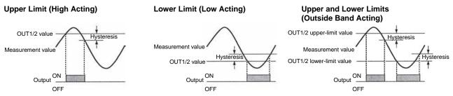
The three types of output operations shown above can be combined as desired. The following are examples of possible combinations.
