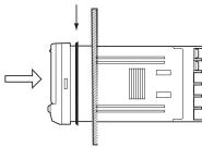
Fit the adaptor into the grooves on the left and right sides of the rear case, then push it until it contacts the panel to secure the K3MA-J.
