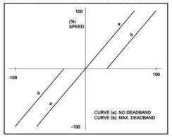
Note: If the deadband trimpot is set too low (CCW direction), the motor may oscillate between forward and reverse. Adjust deadband trimpot CW until the instability disappears. (Oscillation may also occur due to response setting. See section VIII, G, p. 15.)
