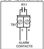
I. Alarm Contacts – S.P.S.T. relay contacts (terminals "3" and "4") are used to signal a warning or to shut other equipment down if control goes to an Inhibit state. Rating of contacts are 1A-28VDC, .5A-115VAC. See table 8 for relay control state vs contact state. (See fig. 9D, p. 11.)
