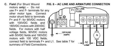
CAUTION – Shunt-Wound motors may be damaged if field remains connected without motor rotating for an extended period of time.
