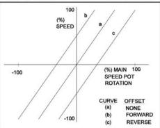
FIG. 12 - DEADBAND TRIMPOT ADJUSTMENT
