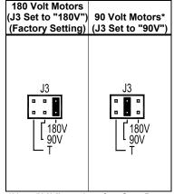
\*Use "90V" setting for Step-Down Operation (90 Volt DC Motors with 208/230 Volt AC Line input).
