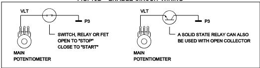
Note: The MIN speed trimpot must not be set higher then 70% CW rotation (approx. 2:00 o'clock position) or Enable will not function.
