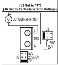
Note: If tach-generator feedback is not required, the position of Jumper J3 does not matter.
