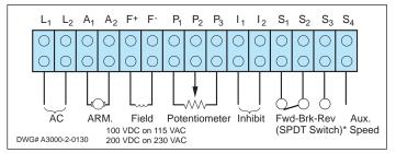
Note: Only 10 mA of current is switched. Any switch or relay may be used except a solid state type or a relay with capacitors or R-C networks (snubbers) across its contacts.
