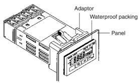
The H8GN's panel surface is water-resistive (conforming to NEMA 4X (indoors) and IP66). In order to prevent the internal circuit from water penetration through the space between the Counter and operating panel, attach a rubber packing (provided with the H8GN) between the Counter and operating panel and secure the rubber packing with the Y92F-34 Flush-mounting Adaptor.
