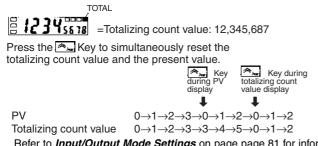
Refer to *Input/Output Mode Settings* on page page 81 for information on totalizing counter operation.
