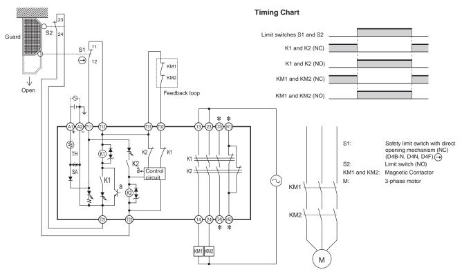
**Note:** External connections and timing charts for G9SB-200-B/301-B models are the same as those for G9SB-2002-A/3012-A models. **\*** Only the G9SB-3012-A model has terminals 33-34 and 41-42.
