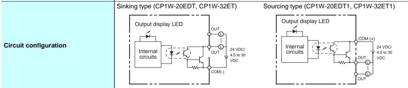
\*1. A maximum of 0.9 A per common can be switched at an ambient temperature of 50°C.
