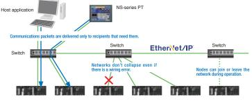
Star topology using Ethernet switch technology
