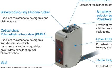
The seal provides the durability to high-temperature and high-pressure water that complies with IP69K.
