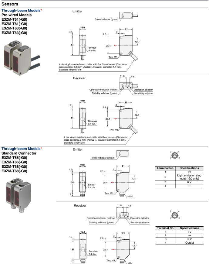
\* Models numbers for Through-beam Sensors (E3ZM-T□□(-G0)) are for sets that include both the Emitter and Receiver. The model number of the Emitter is expressed by adding "-L" to the set model number (example: E3ZM-T61-L 2M, E3ZM-T61-G0-L 2M), the model number of the Receiver, by adding "-D" (example: E3ZM-T61-D 2M, E3ZM-T61-G0-D 2M.) Refer to Ordering Information to confirm model numbers for Emitter and Receivers.
