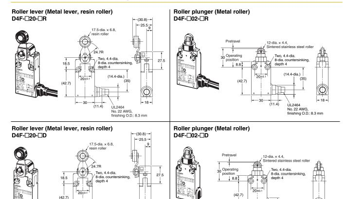
Note: Each dimension has a tolerance of 0.4 mm unless otherwise specified.
