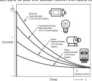
Before using the Switch, be sure to test the Switch under actual conditions. This product is a standard load type Switch. Using the Switch for opening and closing a microload circuit may cause contact failure. Use the Switch within the operating range as shown in below chart.
