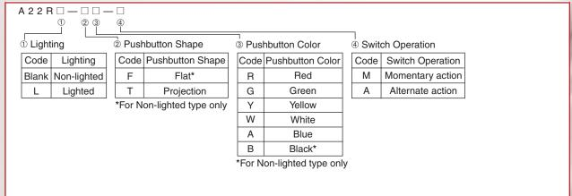
■ Individual unit (Selector unit) A22R□-□□ Selector switches
