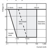
When use the Switch for opening and closing a microload or large-load, use the Switch with an appropriate relay.
