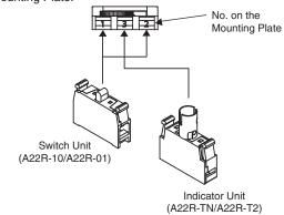
Hook the small protrusion on the Switch Block into the groove on the Mounting Latch on the other side of the lever, then push up the Switch Block in the direction indicated by the arrow in the figure below: • One more Switch Block can be mounted.
