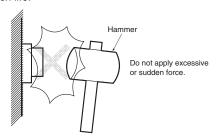
The pushbutton surface is composed of resin. Therefore, do not attempt to operate the pushbutton using a sharp object, such as a screwdriver or a pair of tweezers. Also, do not drop, throw, or knock the Switch. Doing so may damage or deform the pushbutton surface and result in faulty operation.
