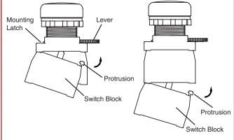
Note: In case that two Switch Block are mounted, a Control Box cannot be used.
