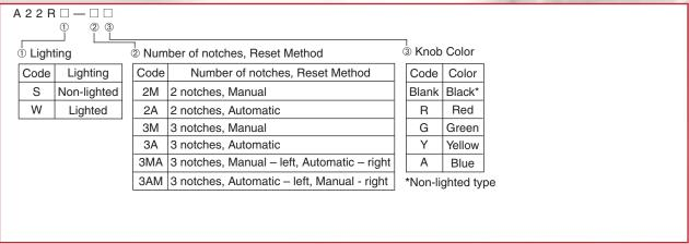
Individual unit (Key selector unit) A22RK-□ Key selector switches
